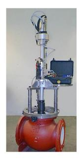
**Repairing leaking valves** in industrial pipelines is a laborious operation involving extended downtime, production losses and substantial, unwanted costs.
